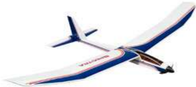
Remote Sensing (Vis/NIR) and Atmospheric Profiling (T/RH/P) UAV
